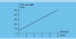
Note: test carried out with a 2 mm inner diameter tube.
