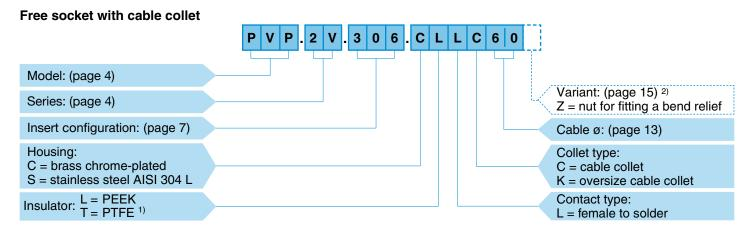
**PVP.2V.306.CLLC60** = free socket with cable collet, 2V series, multipole type with 6 contacts, outer shell in chrome-plated brass, PEEK insulator, female solder contacts, C type collet for 6 mm diameter cable.
