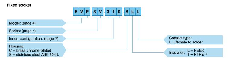
**EVP.3V.310.SLL** = fixed socket, nut fixing, 3V series, multipole type with 10 contacts, outer shell in stainless steel, PEEK insulator, female solder contacts.
