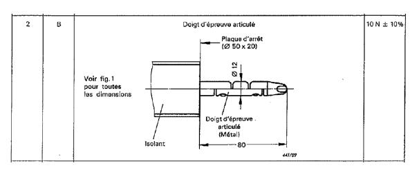
Figure 2, above shows the test probe to be used during test section BP5
