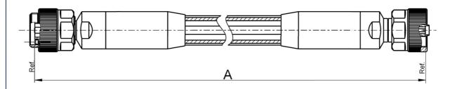
All dimensions are in mm; tolerances:  $\pm$  3mm for A  $\leq$  300 mm;  $\pm$  1% for A > 300 mm
