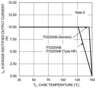
Figure 4. DC Forward Current Derating
