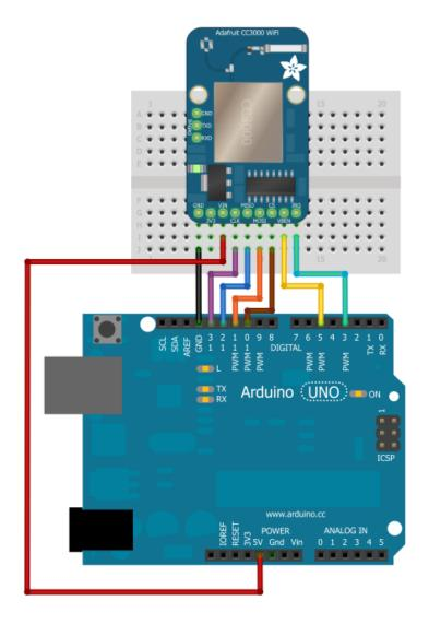
3.3v is an output from the breakout board's voltage regulator - we won't be connecting anything to it in this tutorial.
