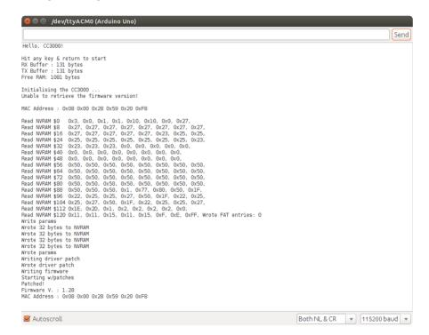
After the upgrade finishes load the buildtest example and run it again. Confirm that everything works as expected with the connection to your wireless network and ping of adafruit.com. Congratulations you've upgraded the firmware on the CC3000!
