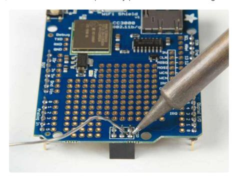
By default, SPI through the ICSP header is not connected. To enable the ICSP header connections, you'll have to connect three solder jumpers on the bottom of the
