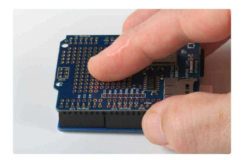
Place the shield over the pins, and carefully solder each one in place (see our <u>Guide To Excellent Soldering</u> (https://adafru.it/aTk) for instructions and tips on getting the best results).
