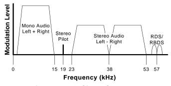
Figure 8. MPX Signal Spectrum
