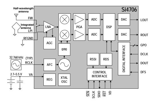
Figure 7. Functional Block Diagram
