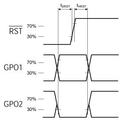
Figure 1. Reset Timing Parameters for Busmode Select Method
