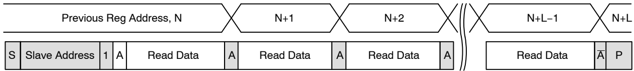
Figure 38. Single READ from Current Location
