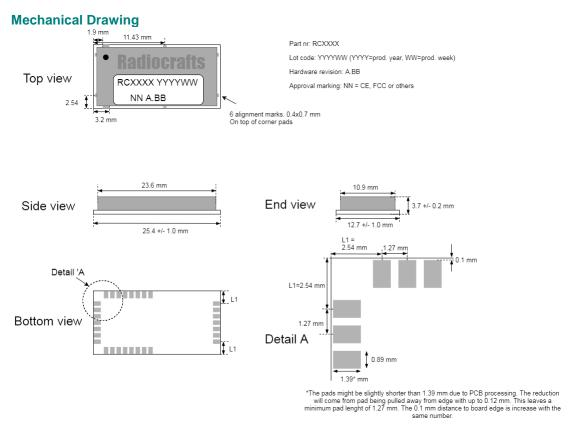
Alignment marking: On the top side there are 8 alignment markers which align with the corresponding pad on the bottom side.
