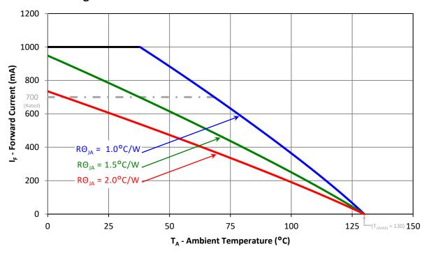
Figure 10: Maximum forward current vs. ambient temperature based on  $T_{J(MAX)}$  = 130°C.
