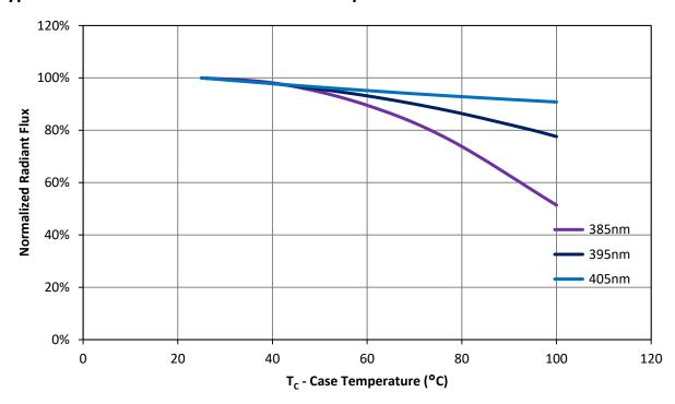
Figure 8: Typical normalized radiant flux vs. case temperature @700mA
