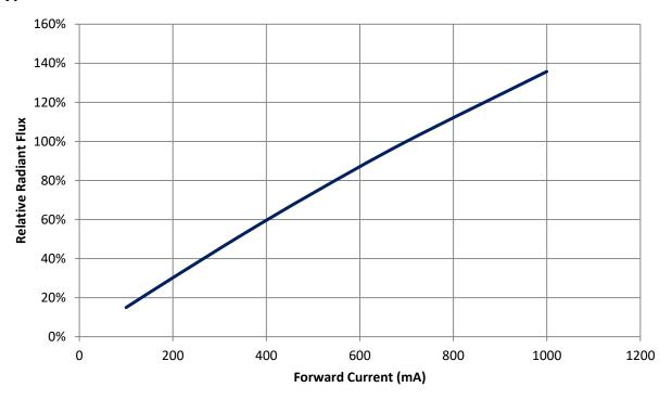
Figure 7: Typical normalized radiant flux vs. forward current @  $T_{\rm C}$  = 25°C.
