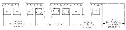
Figure 11: Emitter carrier tape specifications (mm).
