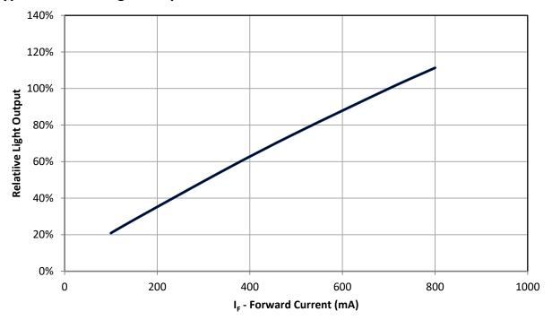
Figure 7: Typical relative light output vs. forward current @  $T_{\text{C}}$  = 25°C.
