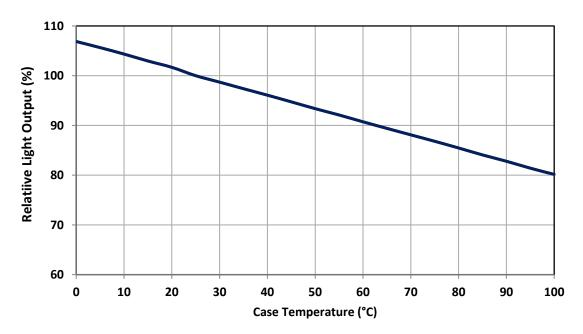
Figure 8: Typical relative light output vs. case temperature.
