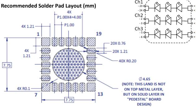
Figure 2a: Recommended solder pad layout for anode, cathode, and thermal pad.
