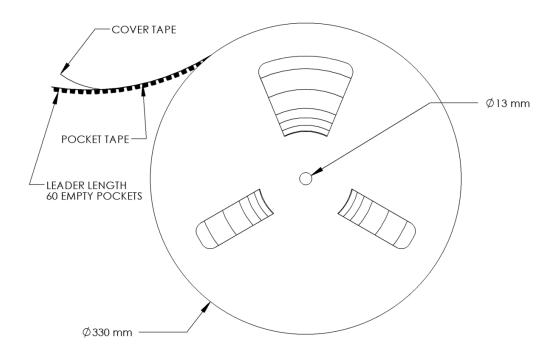
Figure 12: Emitter Reel specifications (mm).
