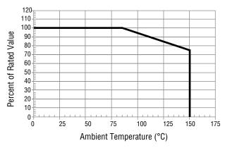
This graph shows the typical device surge current derating versus ambient temperature when subjected to the 8/20 µs current waveform per the IEC 61000-4-5 specification. This device is not intended for continuous operation at temperatures above 125 °C.
