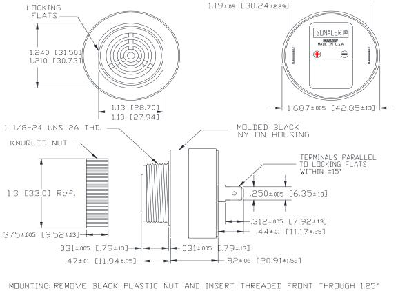
MOUNTING: REMOVE BLACK PLASTIC NUT AND INSERT THREADED FRONT THROUGH 1.25" HOLE PUNCHED IN PANEL, IF ORIENTATION IS NEEDED, NOTE LOCKING FLATS ON DRAWING. SCREW NUT BACK ON. DO NOT OVERTIGHTEN.
