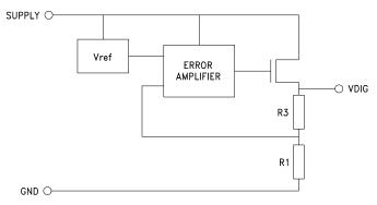
Figure 1. Low Voltage Linear Regulator (VDIG) Block Diagram
