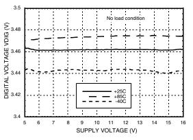
**VDRAIN Load Regulation Over Vdd**
