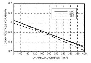
VNEG Load Regulation Over Temperature [2]
