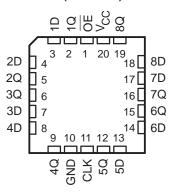
The output enable  $(\overline{OE})$  input does not affect internal operations of the flip-flop. Old data can be retained or new data can be entered while the outputs are in the high-impedance state.
