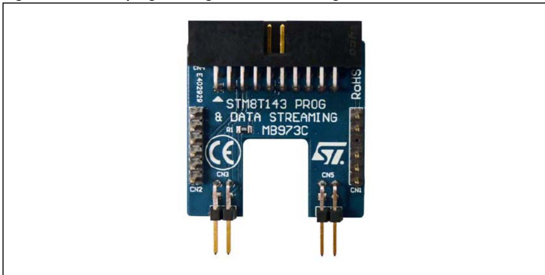
Figure 4. MB973 programming and data streaming board
