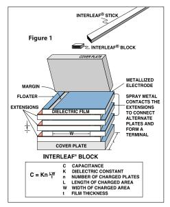
assembly. There exist no metal leaching or dielectric diffusion mechanisms to affect the reliability over time. A complete reliability data package on this and other quality MLP capacitor styles may be obtained by contacting Paktron.
