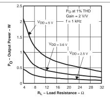
Figure 36. Output Power versus Load Resistance
