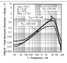
Figure 15. Total Harmonic Distortion + Noise versus Frequency
