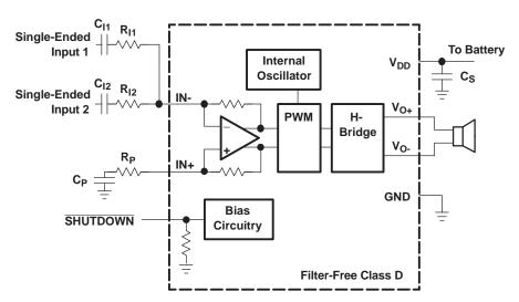
Figure 33. TPA2010D1 Summing Two Single-Ended Inputs
