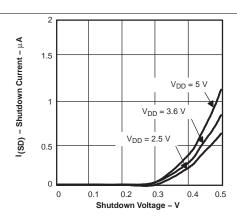
Figure 8. Supply Current versus Shutdown Voltage
