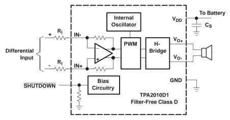
Figure 34. TPA2010D1 with Differential Input
