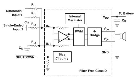
Figure 32. TPA2010D1 Summing Differential Input and Single-Ended Input Signals
