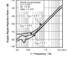
Figure 19. Supply Ripple Rejection Ratio versus Frequency
