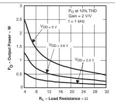
Figure 9. Output Power versus Load Resistance
