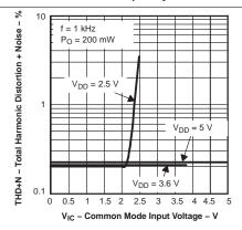
Figure 18. Total Harmonic Distortion + Noise versus Common Mode Input Voltage
