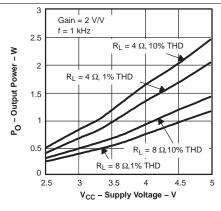
Figure 11. Output Power versus Supply Voltage
