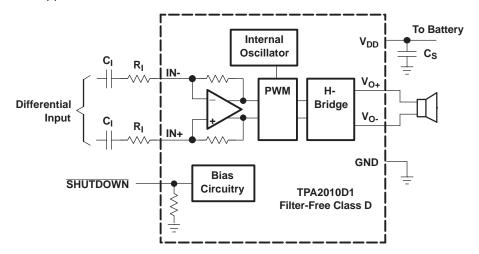
Figure 38. TPA2010D1 With Differential Input and Input Capacitors
