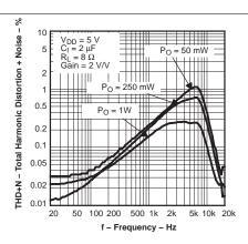
Figure 14. Total Harmonic Distortion + Noise versus Frequency
