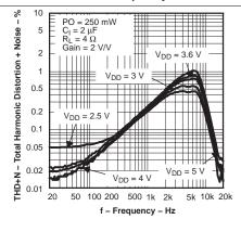
Figure 17. Total Harmonic Distortion + Noise versus frequency
