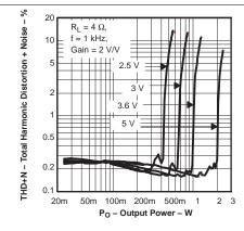
Figure 12. Total Harmonic Distortion + Noise versus Output Power
