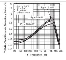
Figure 16. Total Harmonic Distortion + Noise versus Frequency
