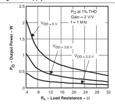
Figure 10. Output Power versus Load Resistance
