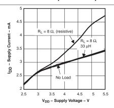
Figure 7. Supply Current versus Supply Voltage
