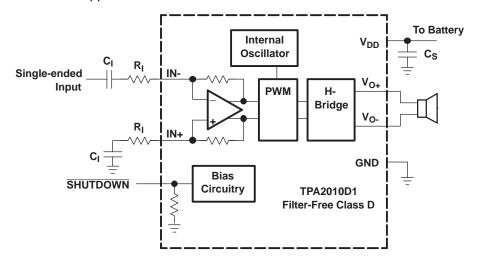
Figure 39. TPA2010D1 with Single-Ended Input
