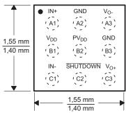
Note: Pin A1 is marked with a "0" for Pb-free (YZF) and a "1" for SnPb (YEF).
