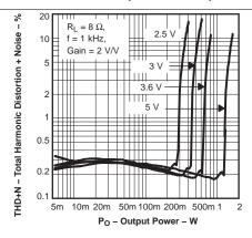
Figure 13. Total Harmonic Distortion + Noise versus Output Power
