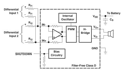
Figure 31. TPA2010D1 Summing Two Differential Inputs
