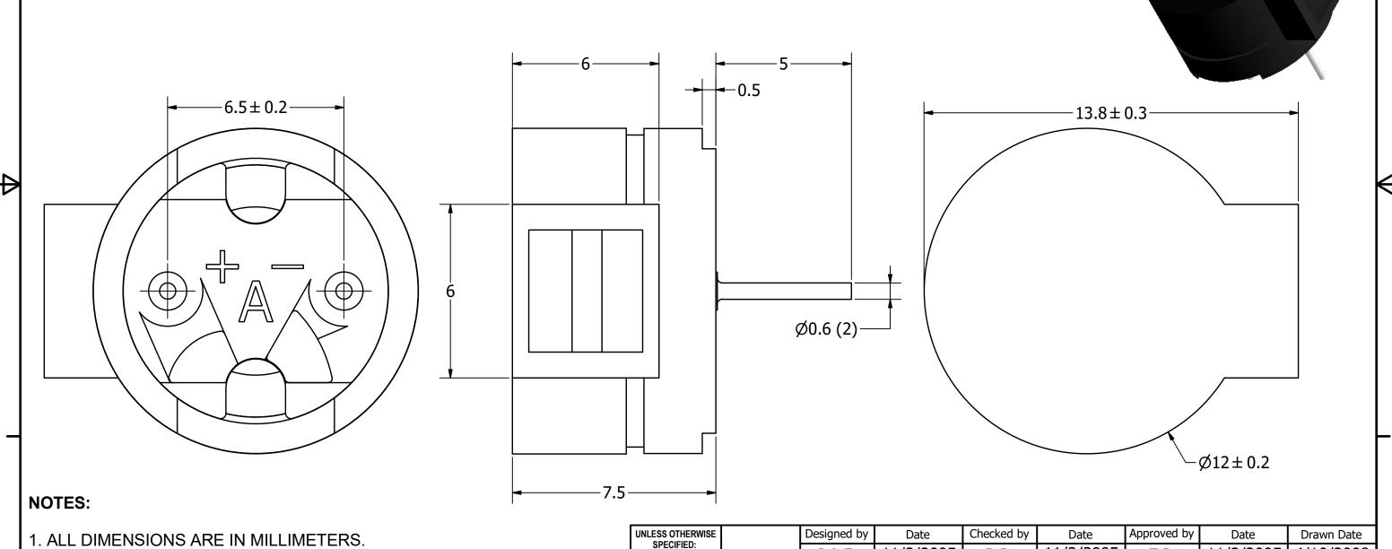
DIMENSIONS ARE IN MILLIMETERS,
