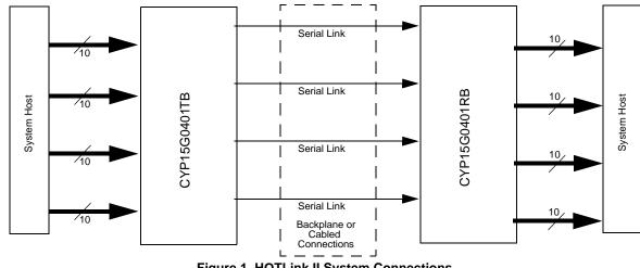
Figure 1. HOTLink II System Connections
