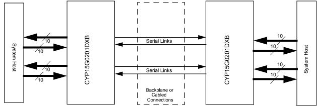
Figure 1. HOTLink II™ System Connections
