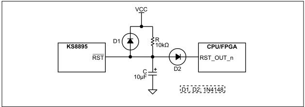
At power-on-reset, R, C, and D1 provide the necessary ramp rise time to reset the device. The reset out RST\_OUT\_n from CPU/FPGA provides the warm reset after power-up.
