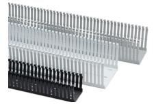
High Density Slotted Wall Wiring Duct, 2" x 2", Non-Adhesive, PVC, Gray, 120ft/Carton
