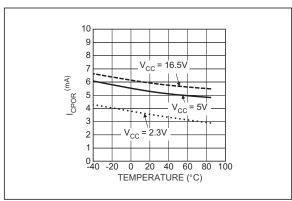
**FIGURE 2-3:** Power-On Reset Timer (Off) Current vs. Temperature.
