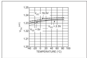
FIGURE 2-12: POR Delay/Overcurrent Timer Threshold vs. Temperature.
