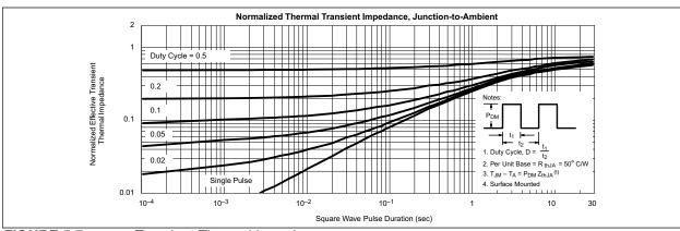
FIGURE 5-7: Transient Thermal Impedance
