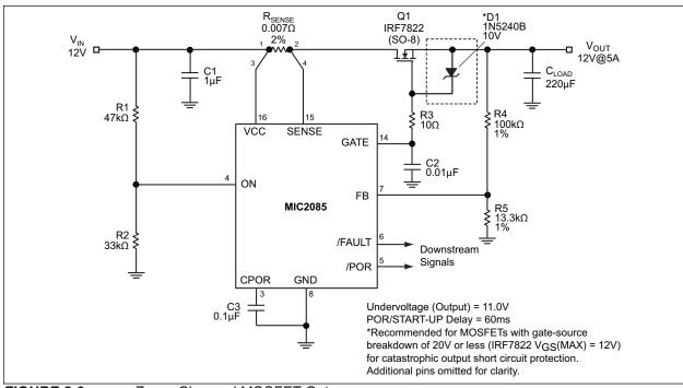
FIGURE 5-6: Zener-Clamped MOSFET Gate.
