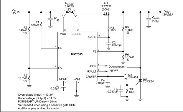
FIGURE 5-1: Undervoltage/Overvoltage Circuit.
