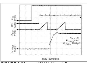
FIGURE 2-23: 12V Hot Insert Response.
