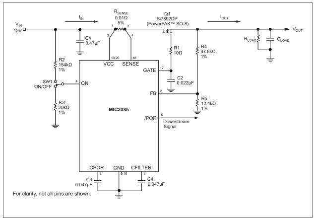
FIGURE 2-29: Test Circuit.
