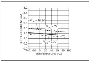
FIGURE 2-1: Supply Current vs. Temperature.
