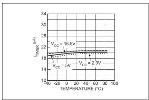
**FIGURE 2-4:** Overcurrent Timer Current vs. Temperature.
