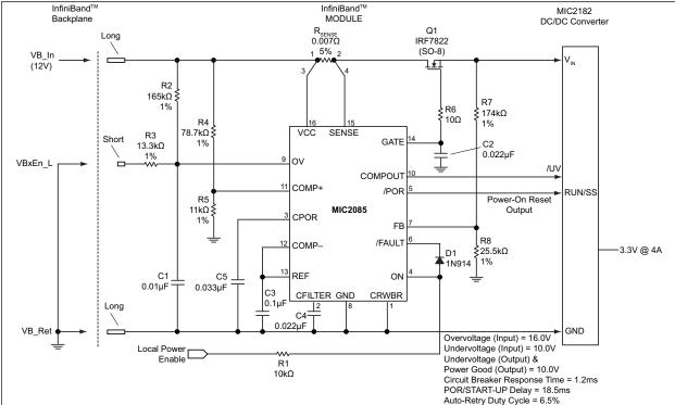
FIGURE 5-5: A 50W InfiniBand™ Application.
