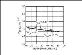
FIGURE 2-14: Current Limit Threshold (Slow Trip) vs. Temperature.
