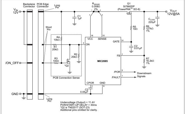
FIGURE 5-2: PCB Connection Sense with ON/OFF Control.
