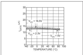
FIGURE 2-6: Gate Pull-Up Current vs. Temperature.
