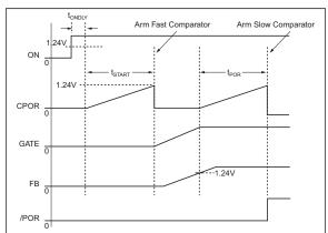
FIGURE 1-3: Power-On Start-Up Delay Timing.
