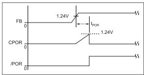
FIGURE 1-2: Power-On Reset Response.
