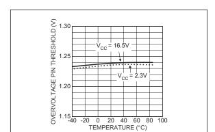
FIGURE 2-20: vs. Temperature.
