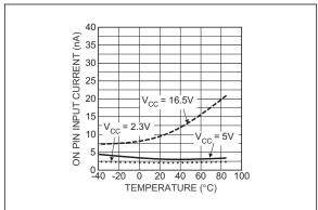
**FIGURE 2-18:** ON Input Current vs. Temperature.
