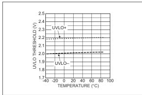
FIGURE 2-15: UVLO Threshold vs. Temperature.
