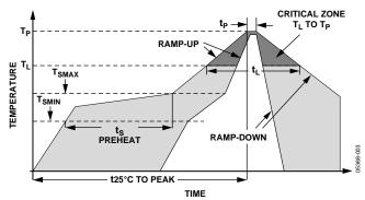
Figure 3. Recommended Soldering Profile
