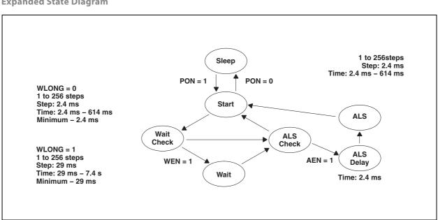
Figure 20: Expanded State Diagram
