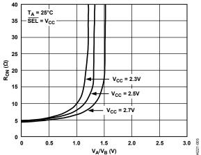
Figure 5. On Resistance vs. Input Voltage
