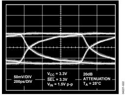
Figure 22. Eye Pattern; 1.5 Gbps,  $V_{CC} = 3.3 V$ , PRBS 31
