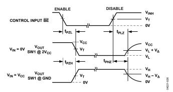
Figure 26. Enable and Disable Times
