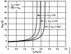
Figure 4. On Resistance vs. Input Voltage
