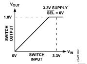
Figure 33. 3.3 V to 1.8 V Voltage Translation,  $\overline{SEL} = 0 \text{ V}$
