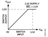
Figure 29. 3.3 V to 2.5 V Voltage Translation,  $\overline{SEL} = V_{CC}$
