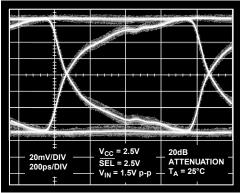
Figure 23. Eye Pattern; 1.244 Gbps,  $V_{CC} = 2.5 V$ , PRBS 31
