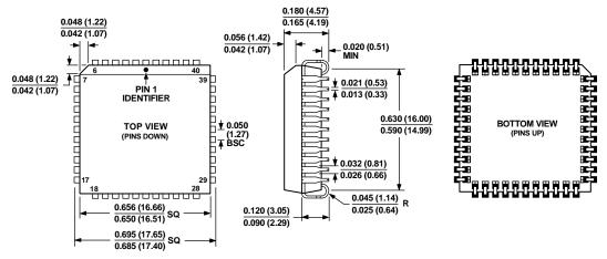
COMPLIANT TO JEDEC STANDARDS MO-047-AC CONTROLLING DIMENSIONS ARE IN INCHES; MILLIMETER DIMENSIONS (IN PARENTHESES) ARE ROUNDED-OFF INCH EQUIVALENTS FOR REFERENCE ONLY AND ARE NOT APPROPRIATE FOR USE IN DESIGN.
