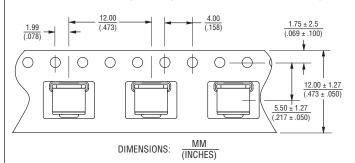
Unless otherwise specified, tolerances in decimals are .X  $\pm$  0.3, .XX  $\pm$  0.15 for lengths in millimeters and  $\pm$ 1 ° for degrees.
