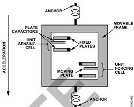
Figure 5. Simplified View of Sensor Under Acceleration
