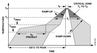
Figure 3. Recommended Soldering Profile
