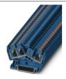
Feed-through terminal block, Connection method: Push-in connection, Cross section: 0.2 mm<sup>2</sup> - 6 mm<sup>2</sup>, AWG: 24 - 10, Width: 6.2 mm, Color: blue, Mounting type: NS 35/7,5, NS 35/15
