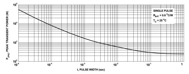
Figure 11. Single Pulse Maximum Power Dissipation
