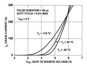
Figure 5. Transfer Characteristics
