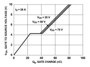
Figure 7. Gate Charge Characteristics
