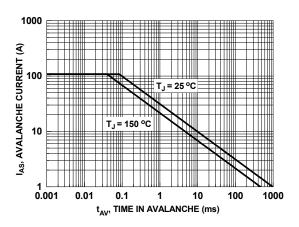
Figure 9. Unclamped Inductive Switching Capability
