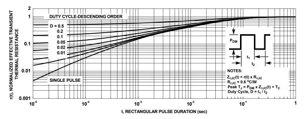
Figure 12. Junction-to-Case Transient Thermal Response Curve
