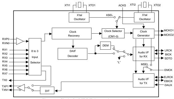
Figure 16. Clocks for DIT/DIR in asynchronous mode
