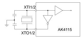
Note: External capacitance depends upon the crystal oscillator (typ. 5-10pF)
