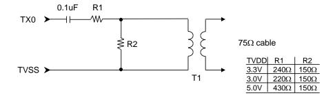
Figure 24. TX0 External Resistor Network 2
