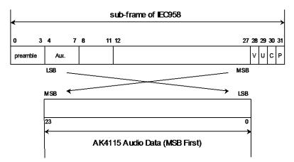
Figure 34. Bit configuration
