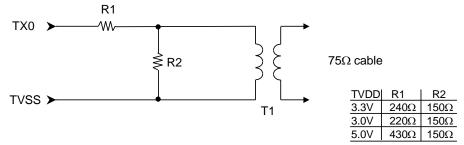
Figure 23. TX0 External Resistor Network 1
