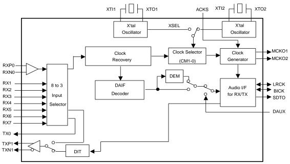
Figure 14. Clocks for DIT/DIR in synchronous mode (PSEL bit = "0")
