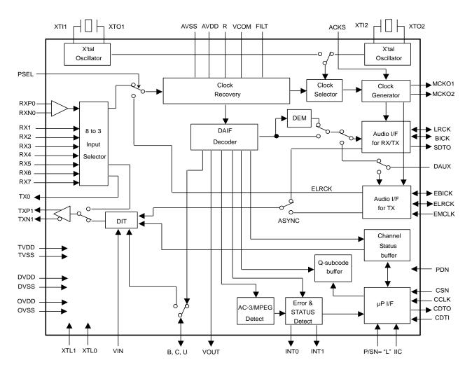
Figure 1. AK4115 Block Diagram in serial mode
