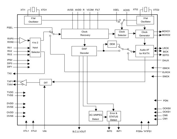
Figure 2. AK4115 Block Diagram in parallel mode
