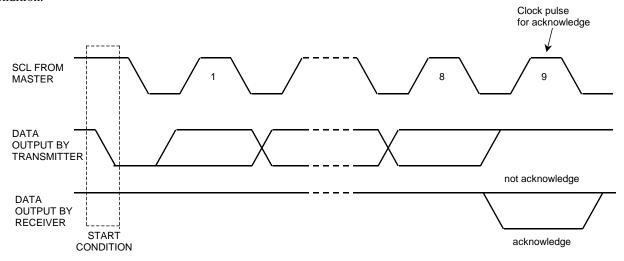
Figure 43. Acknowledge on the I<sup>2</sup>C-bus
