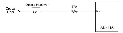
Figure 22. Consumer Input Circuit (Optical Input)
