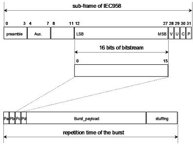
Figure 50. Data structure in IEC60958
