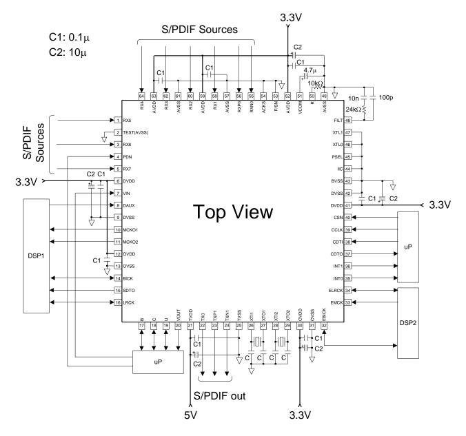
Figure 53. Typical Connection Diagram (4-wire serial mode)
