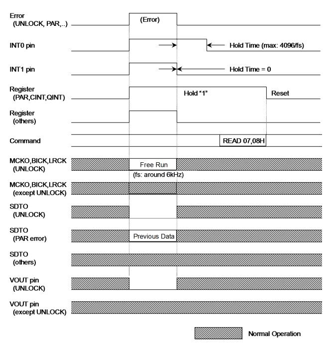
Figure 31. INT0/1 pin timing
