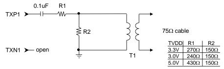
Figure 26. Consumer Output Driver Circuit at AC coupling
