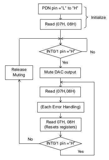
Figure 32. Error Handling Sequence Example 1
