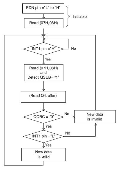
Figure 33. Error Handling Sequence Example (for Q/CINT)
