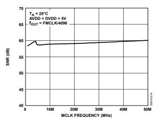
Figure 14. SNR vs. MCLK Frequency
