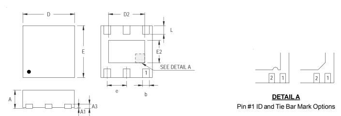
Note: The configuration of the Pin#1 identifier is optional, but must be located within the zone indicated.
