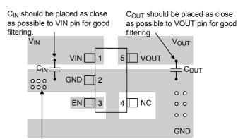
The through hole of the GND pin is recommended to be as many as possible.
