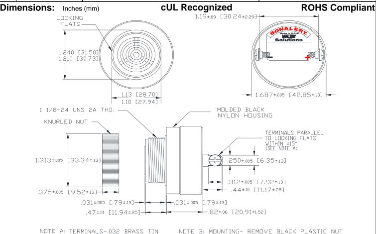
AND INSERT THREADED FRONT THROUGH 1.25" HOLE PUNCHED IN PANEL, IF PLATED, TAPPED FOR #6-32 SCREW. TWO #6-32 NICKEL PLATED BRASS SCREWS DRIENTATION IS NEEDED, NOTE LOCKING FLATS ON DRAWING, SCREW NUT BACK ON, DO NOT OVERTIGHTEN. INCLUDED. WILL ACCEPT 1/4" QUICK CONNECT.
