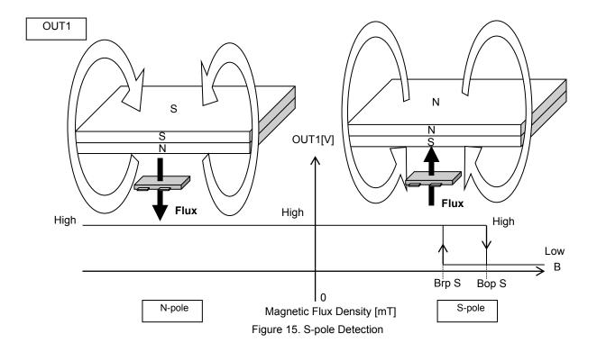
The OUT1 pin detects and outputs for the S-pole only. Since the OUT1 pin output is unipolar, the output does not respond to the N-pole.
