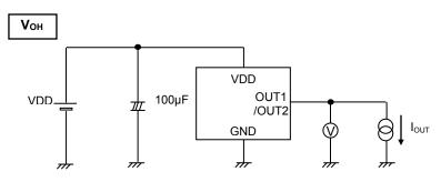
Figure 3. V<sub>OH</sub> Measurement Circuit
