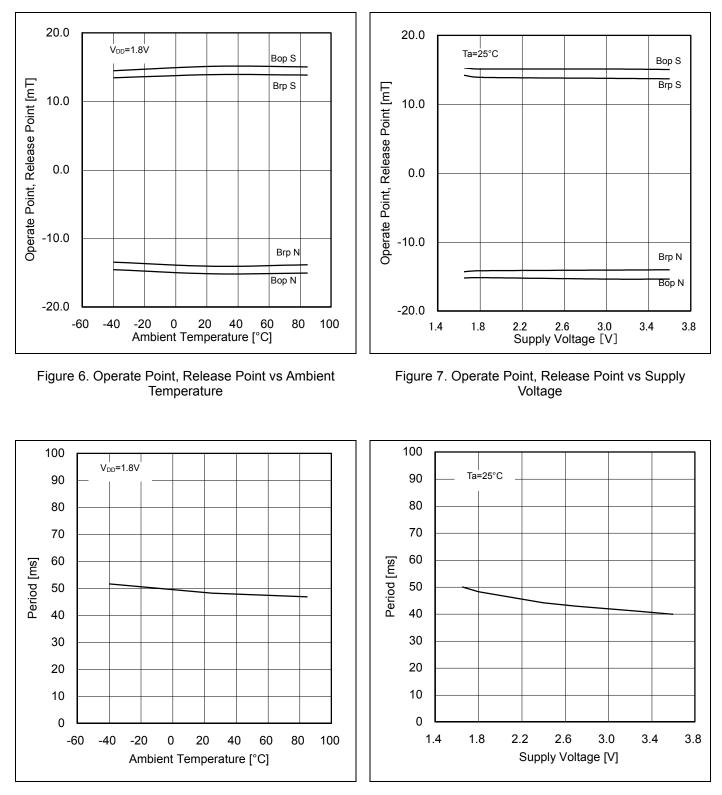
Figure 9. Period vs Supply Voltage
