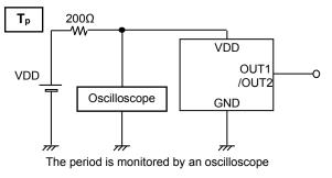
Figure 2. Tp Measurement Circuit
