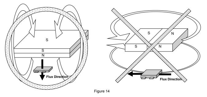
The Hall IC cannot detect magnetic fields that run horizontal to the package top layer. Be certain to configure the Hall IC so that the magnetic field is perpendicular to the top layer.
