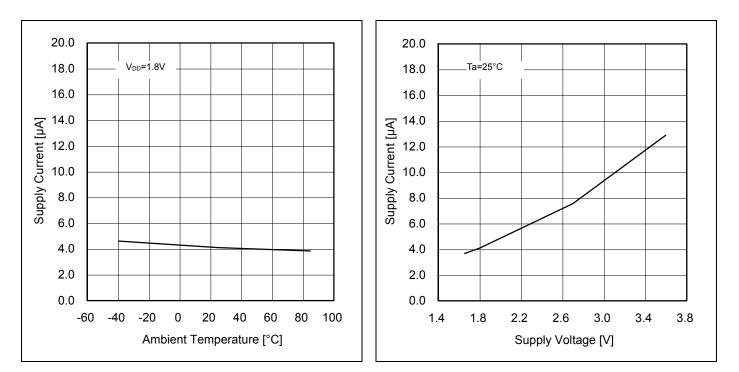
Figure 10. Supply Current vs Ambient Temperature
