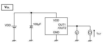
Figure 4. VoL Measurement Circuit
