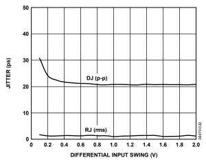
Figure 20. Jitter vs. Differential Input Swing
