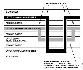
Figure 32. Example Routing of Reference Plane
