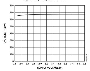
Figure 19. Eye Height vs. Supply Voltage
