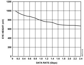
Figure 18. Eye Height vs. Data Rate
