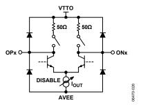
Figure 26. High Speed Output Simplified Schematic
