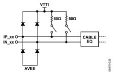
Figure 25. High Speed Input Simplified Schematic
