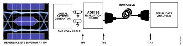
Figure 9. Test Circuit Diagram for TX Eye Diagram
