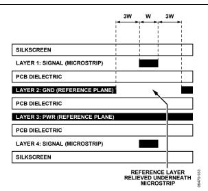
Figure 33. Example Board Stackup
