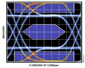
Figure 11. TX Eye Diagram at TP2, PE = 6 dB
