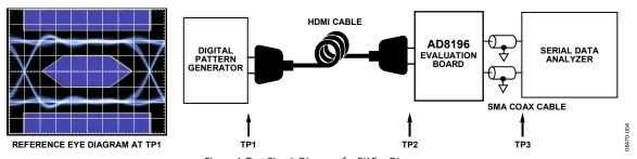
Figure 4. Test Circuit Diagram for RX Eye Diagrams
