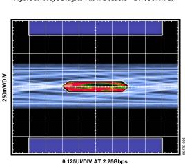
Figure 6. RX Eye Diagram at TP2 (Cable = 20 m, 24 AWG)
