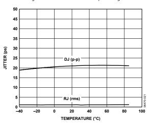
Figure 21. Jitter vs. Temperature
