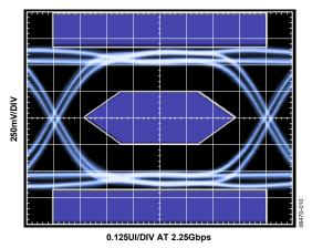
Figure 10. TX Eye Diagram at TP2, PE = 2 dB
