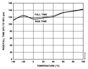
Figure 22. Rise and Fall Time vs. Temperature
