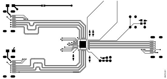
Figure 31. Evaluation Board Layout of the TMDS Traces
