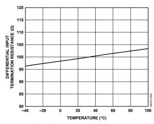
Figure 24. Differential Input Termination Resistance vs. Temperature
