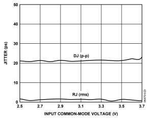
Figure 23. Jitter vs. Input Common-Mode Voltage
