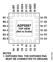
Figure 3. LFCSP Pin Configuration
