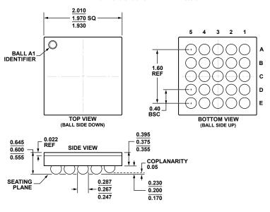
Figure 22. 25-Ball Wafer Level Chip Scale Package [WLCSP] (CB-25-4) Dimensions shown in millimeters
