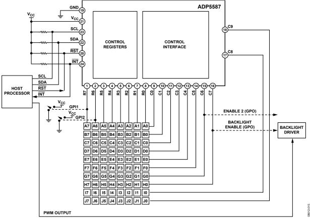
Figure 19. ADP5587 Detailed Application Block Diagram
