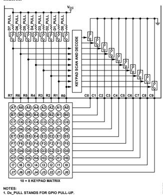
Figure 10. Keypad Decode Configuration
