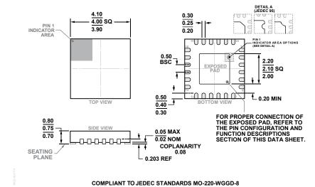
Figure 21. 24-Lead Lead Frame Chip Scale Package [LFCSP] 4 mm × 4 mm Body and 0.75 mm Package Height (CP-24-10)
