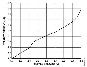
Figure 8. Supply Voltage vs. Standby Current
