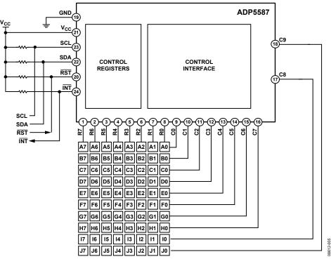
Figure 9. Typical Operating Circuit
