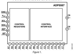
All communication to the main processor is done using one interrupt line and two I $^2$ C-compatible interface lines. The ADP5587 can be configured as a keypad matrix of up to 8 rows  $\times$  10 columns (a maximum of 80 keys).
