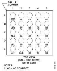
Figure 4. WLCSP Pin Configuration
