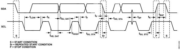
Figure 2. I<sup>2</sup>C Interface Timing Diagram
