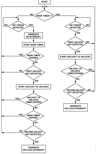
Figure 12. Keypad Lock Interrupt Mask Timer Flowchart
