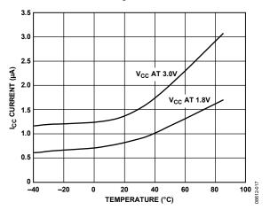
Figure 5. Standby (I<sub>CC</sub>) Current vs. Temperature
