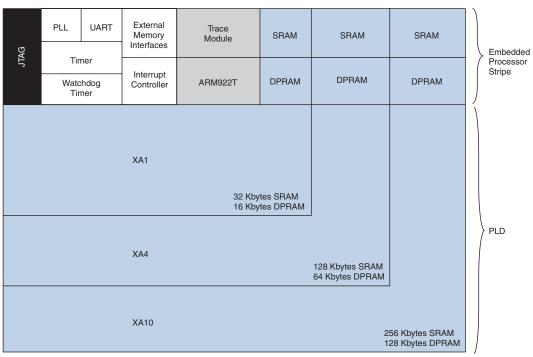
Figure 2. Excalibur System Architecture
