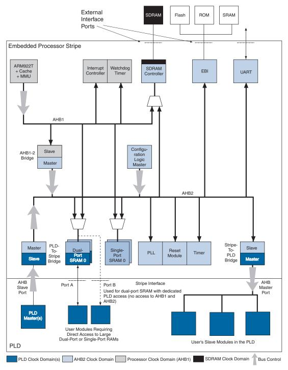
Two AMBA-compliant AHBs ensure that the embedded processor activity is unaffected by peripheral and memory operation. Three bidirectional AHB-to-AHB bridges enable embedded peripherals and PLD-implemented peripherals to exchange data with the embedded processor or with other peripherals.
