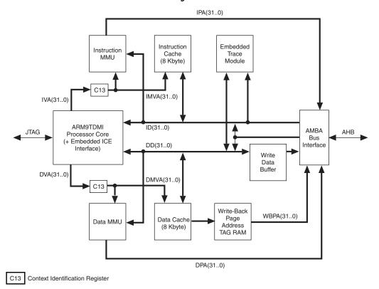
Figure 3. ARM922T Embedded Processor Internal Organization
