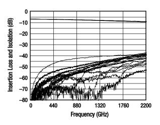
Figure 5. I2 to OUT1 and I2 to OUT2 Paths for States 0 to 15
