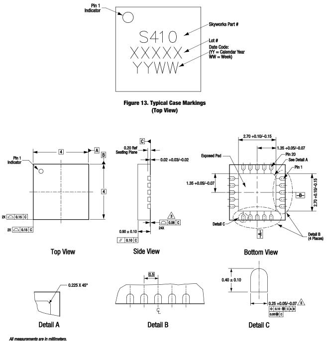
Dimensioning and tolerancing according to ASME Y14.5M-1994.
