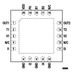
Figure 2. SKY13410-365LF Pinout – 20-Pin QFN (Top View)
