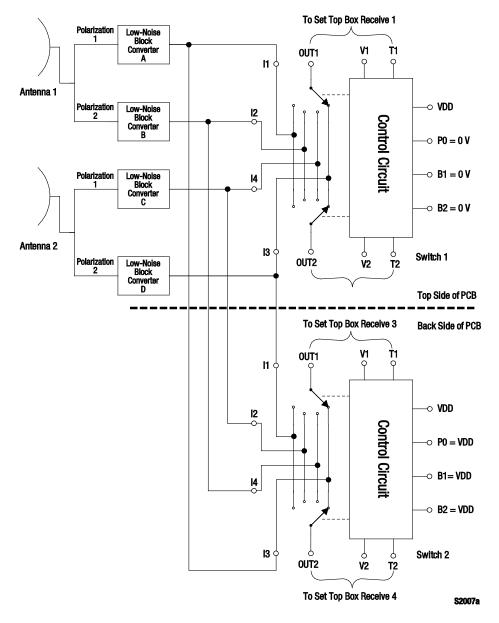
Figure 3. Suggested Implementation of Two 4x2 Switches
