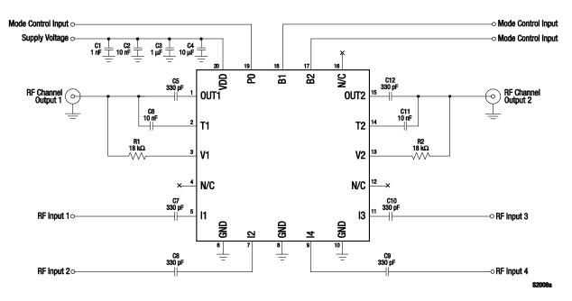
Figure 10. SKY13410-365LF Recommended Application Circuit
