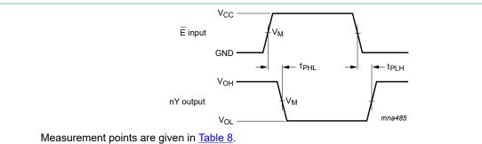
V<sub>OL</sub> and V<sub>OH</sub> are typical voltage output levels that occur with the output load.
