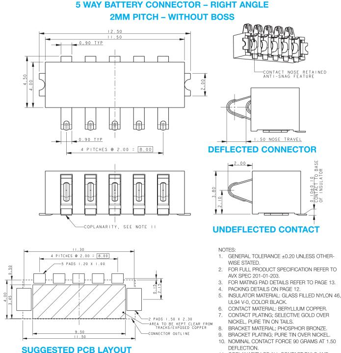
11. COPLANARITY OF ALL CONTACT TAILS AND PADS 0.12MM MAXIMUM.
