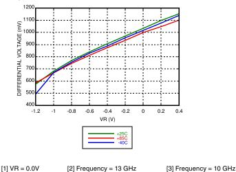
Output Differential vs. Supply Voltage [1] [3]
