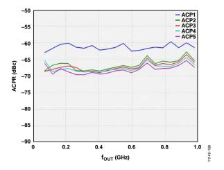
Figure 52. Eight-Carrier ACPR vs. fout
