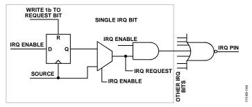
Figure 141. Interrupt Request Circuitry
