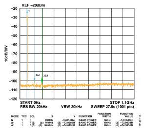
Figure 102. Single Carrier at 70 MHz Output
