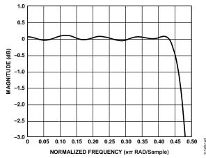
Figure 140. FIR40 2× Interpolation Filter Plot, Pass-Band Ripple
