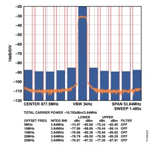
Figure 21. Single-Carrier W-CDMA at 877.5 MHz
