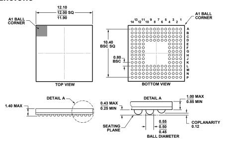
Figure 157. 160-Ball Chip Scale Package Ball Grid Array [CSP\_BGA] (BC-160-1)
