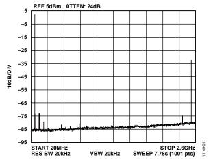
Figure 10. Single-Tone Spectrum at  $f_{OUT} = 70 \text{ MHz}$
