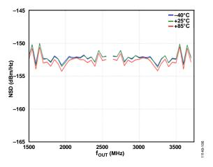
Figure 96. W-CDMA NSD vs. fout over Temperature
