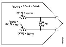
Figure 150. Equivalent DAC Output Circuit
