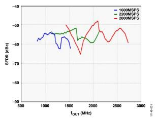
Figure 25. SFDR vs. fout over fdAC
