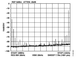
Figure 84. Single-Tone Spectrum at  $f_{OUT} = 2350 \text{ MHz}$
