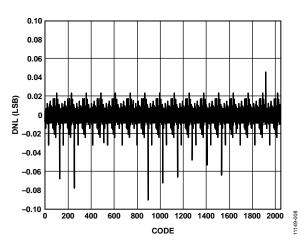
Figure 8. Typical DNL, 22 mA at 25°C
