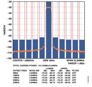
Figure 35. Single-Carrier W-CDMA at 1887.5 MHz
