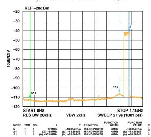
Figure 107. Eight Carrier at 950 MHz Output
