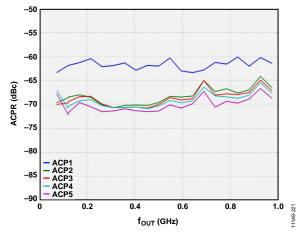
Figure 116. Eight-Carrier ACPR vs. fOUT
