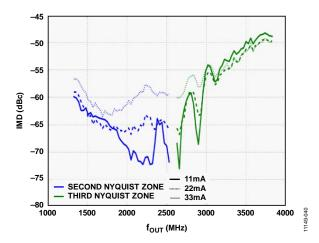
Figure 33. IMD vs.  $f_{\text{OUT}}$  over DAC  $I_{\text{OUTFS}}$
