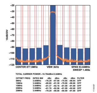
Figure 76. Single-Carrier W-CDMA at 877.5 MHz
