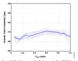
Figure 111. Third Harmonic vs.  $f_{\text{OUT}}$  Performance for One DOCSIS Carrier
