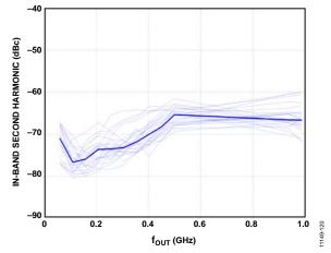
Figure 109. Second Harmonic vs. f<sub>OUT</sub> Performance for Four DOCSIS Carriers
