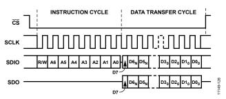
Figure 123. Serial Register Interface Timing, MSB-First Read
