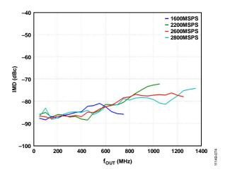
Figure 66. IMD vs. fout over fdac
