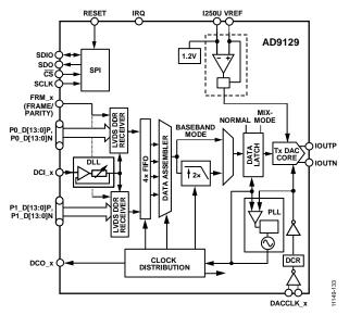
Figure 128. Functional Block Diagram of the AD9119/AD9129
