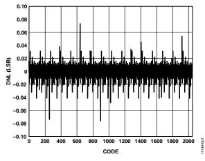
Figure 7. Typical DNL, 11 mA at 25°C
