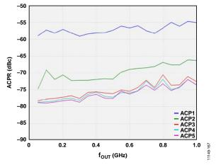
Figure 50. Single-Carrier ACPR vs.  $f_{OUT}$
