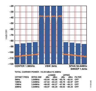
Figure 37. Four-Carrier W-CDMA at 1980 MHz
