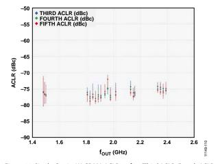
Figure 99. Single-Carrier W-CDMA ACLR vs. f<sub>OUT</sub> (Third ACLR, Fourth ACLR, Fifth ACLR)
