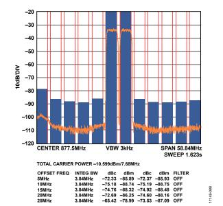
Figure 79. Two-Carrier W-CDMA at 875 MHz
