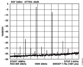
Figure 13. Single-Tone Spectrum at  $f_{OUT} = 1000 \text{ MHz}$
