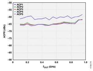
Figure 53. 16-Carrier ACPR vs. f<sub>OUT</sub>
