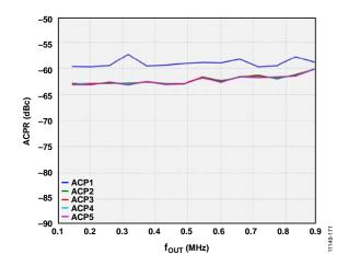
Figure 54. 32-Carrier ACPR vs. fout
