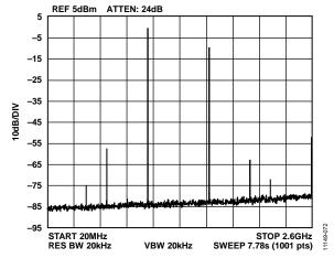
Figure 65. Single-Tone Spectrum at  $f_{OUT} = 1000 \text{ MHz}$
