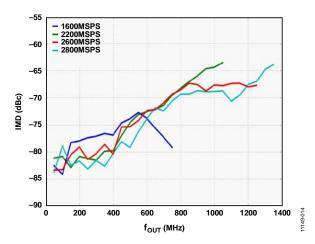
Figure 14. IMD vs. fout over fdac
