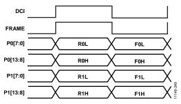
Figure 142. Timing Diagram of FRAME Signal Required to Align Input Data for SED
