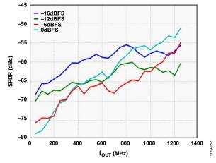
Figure 16. SFDR vs. four over Digital Full Scale
