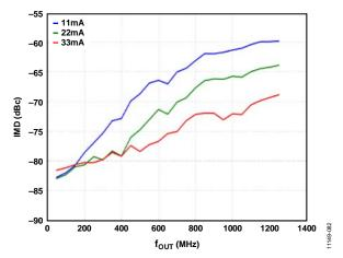
Figure 73. IMD vs. f<sub>OUT</sub> over DAC I<sub>OUTFS</sub>
