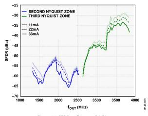
Figure 32. SFDR vs. f<sub>OUT</sub> over DAC I<sub>OUTFS</sub>
