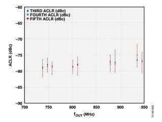
Figure 83. Two-Carrier W-CDMA ACLR vs. fou⊤ (Third ACLR, Fourth ACLR, Fifth ACLR)
