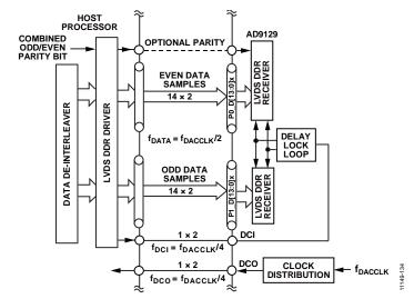
Figure 129. Recommended Digital Interface Between the AD9119/AD9129 and the Host Processor
