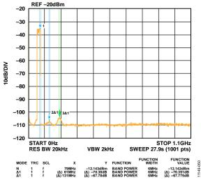
Figure 39. Four Carrier at 70 MHz Output
