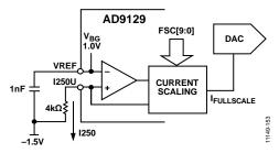
Figure 149. Voltage Reference Circuit
