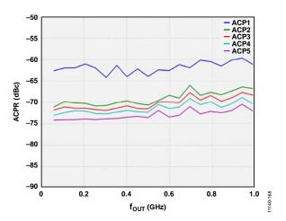
Figure 51. Four-Carrier ACPR vs. four
