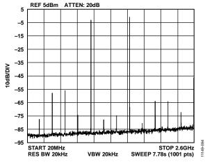
Figure 87. Single-Tone Spectrum at  $f_{OUT} = 1600 \text{ MHz}$
