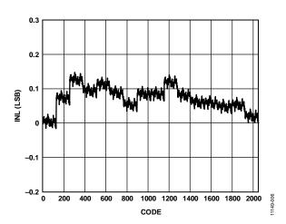
Figure 6. Typical INL, 33 mA at 25  $^{\circ}$ C
