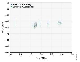
Figure 100. Four-Carrier W-CDMA ACLR vs. fout (First ACLR, Second ACLR)
