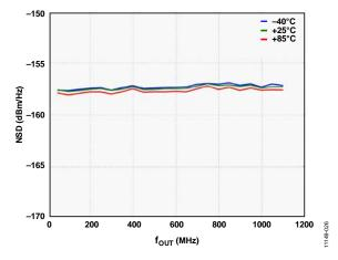
Figure 22. W-CDMA NSD vs. f<sub>OUT</sub> over Temperature
