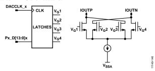
Figure 143. Quad-Switch Architecture
