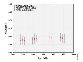
Figure 81. Single-Carrier W-CDMA ACLR vs. f<sub>OUT</sub> (Third ACLR, Fourth ACLR, Fifth ACLR)
