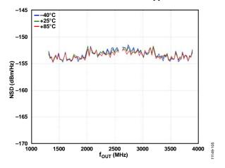
Figure 94. Single-Tone NSD vs. fout over Temperature
