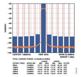
Figure 95. Single-Carrier W-CDMA at 1887.5 MHz
