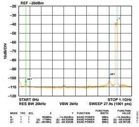
Figure 42. Four Carrier at 950 MHz Output
