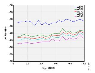
Figure 115. Four-Carrier ACPR vs. fout
