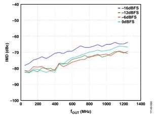
Figure 71. IMD vs.  $f_{OUT}$  over Digital Full Scale
