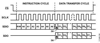
Figure 125. Serial Register Interface Timing, LSB-First Read
