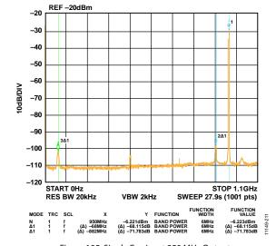
Figure 105. Single Carrier at 950 MHz Output
