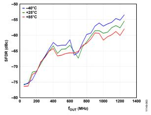
Figure 74. SFDR vs. four over Temperature
