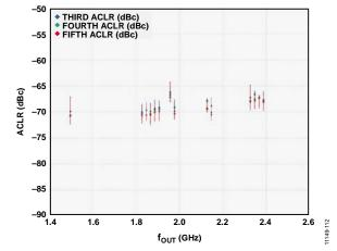
Figure 101. Four-Carrier W-CDMA ACLR vs. f<sub>OUT</sub> (Third ACLR, Fourth ACLR, Fifth ACLR)
