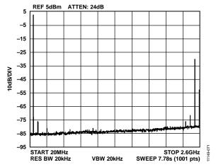
Figure 62. Single-Tone Spectrum at  $f_{OUT} = 70 \text{ MHz}$
