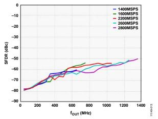
Figure 11. SFDR vs. fout over fDAC
