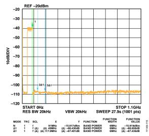
Figure 104. Eight Carrier at 70 MHz Output
