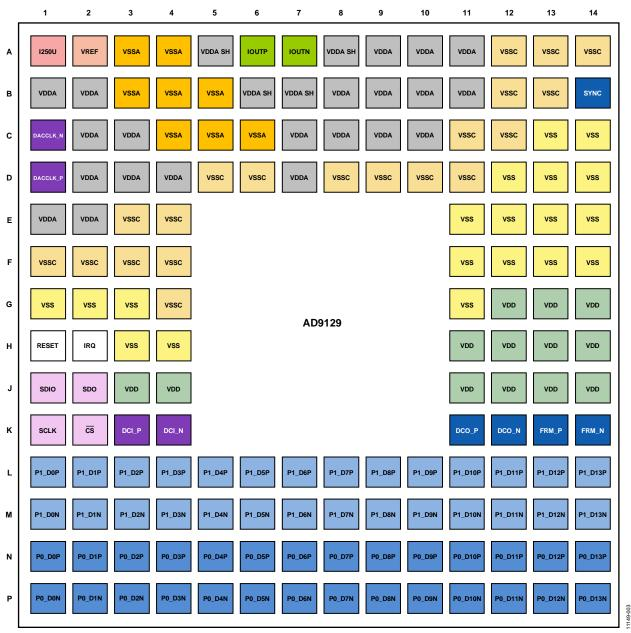
Figure 3. AD9129 Pin Configuration
