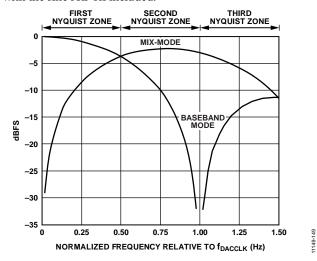
Figure 146. Sinc Roll-Off for Baseband Mode and Mix-Mode Operation
