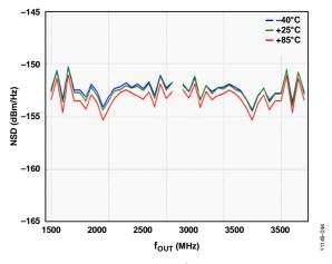
Figure 36. W-CDMA NSD vs. fout over Temperature
