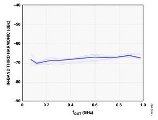
Figure 49. Third Harmonic vs.  $f_{\text{OUT}}$  Performance for Eight DOCSIS Carriers
