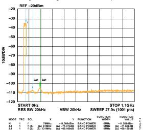
Figure 103. Four Carrier at 70 MHz Output
