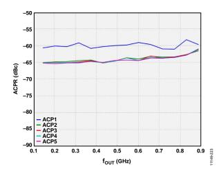
Figure 118. 32-Carrier ACPR vs.  $f_{OUT}$
