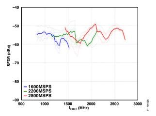
Figure 85. SFDR vs.  $f_{OUT}$  over  $f_{DAC}$
