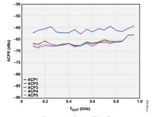
Figure 117. 16-Carrier ACPR vs.  $f_{OUT}$
