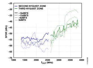
Figure 90. SFDR vs. four over Digital Full Scale
