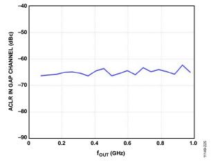
Figure 120. Gap Channel ACLR vs.  $f_{\text{OUT}}$
