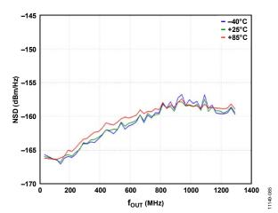
Figure 78. Single-Tone NSD vs. f<sub>OUT</sub> over Temperature
