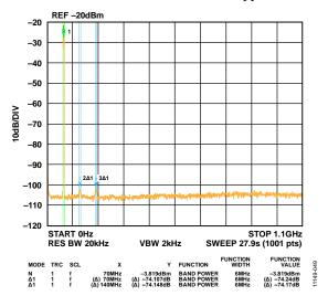
Figure 38. Single Carrier at 70 MHz Output
