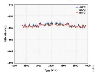
Figure 34. Single-Tone NSD vs.  $f_{\text{OUT}}$  over Temperature
