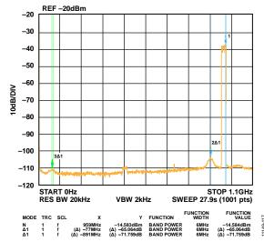
Figure 106. Four Carrier at 950 MHz Output
