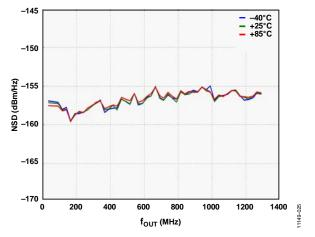
Figure 20. Single-Tone NSD vs. fout over Temperature
