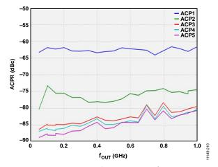
Figure 114. Single-Carrier ACPR vs. fout
