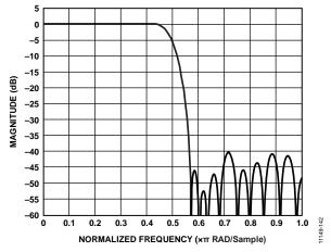
Figure 139. FIR40 2× Interpolation Filter Plot, Complete Frequency Response
