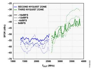
Figure 30. SFDR vs.  $f_{OUT}$  over Digital Full Scale
