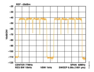
Figure 55. Gap Channel ACPR at 77 MHz
