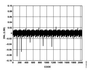
Figure 9. Typical DNL, 33 mA at 25°C
