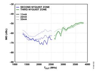
Figure 93. IMD vs. fout over DAC loutes
