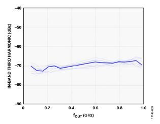
Figure 48. Third Harmonic vs.  $f_{\text{OUT}}$  Performance for Four DOCSIS Carriers
