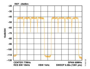
Figure 119. Gap Channel ACLR at 77 MHz
