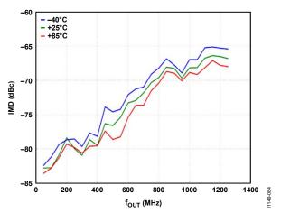
Figure 75. IMD vs.  $f_{OUT}$  over Temperature
