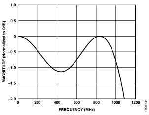
Figure 138. FIR25  $2 \times$  Interpolation Filter Plot, Pass-Band Ripple;  $f_{DAC} = 2.5$  GHz
