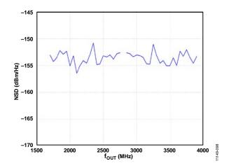
Figure 89. W-CDMA NSD vs. f<sub>OUT</sub>
