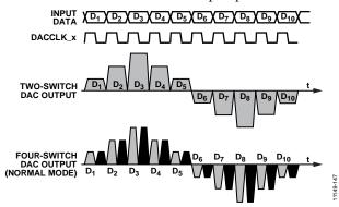
Figure 144. Two-Switch and Quad-Switch DAC Waveforms
