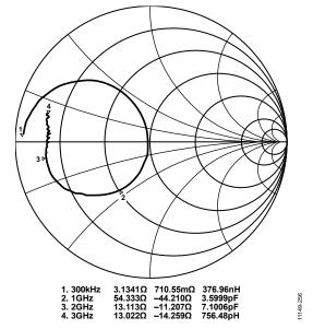
Figure 156. Measured Smith Chart Showing the DAC Output Impedance;  $f_{DAC} = 2.6 \text{ GSPS}$
