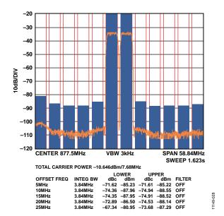
Figure 23. Two-Carrier W-CDMA at 877.5 MHz
