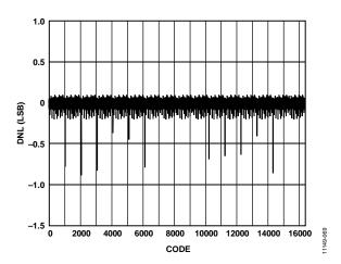
Figure 60. Typical DNL, 22 mA at 25°C
