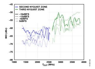
Figure 91. IMD vs.  $f_{OUT}$  over Digital Full Scale
