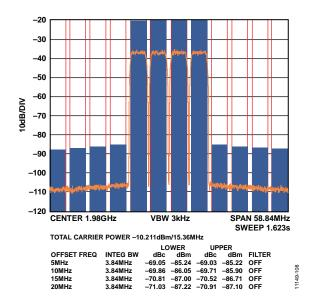
Figure 97. Four-Carrier W-CDMA at 1980 MHz
