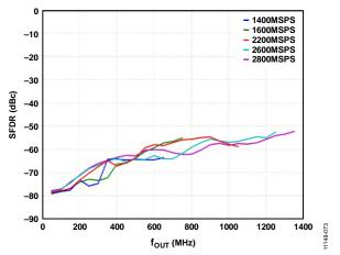
Figure 63. SFDR vs. fout over fdAC
