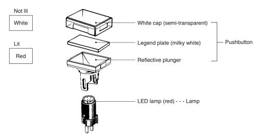
Ordering: With colored-illumination models, order the Pushbutton, Lamp, and Switch as shown in the following table.
