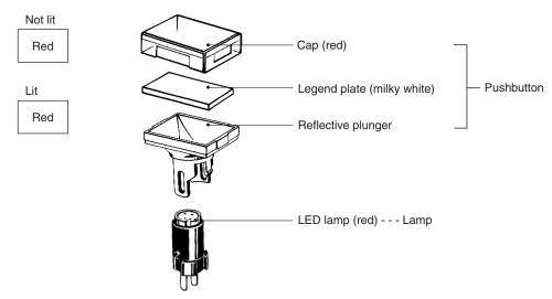
"Colored illumination" describes LED models for which the screen color is white when the LED is not lit and changes to the color of the LED lamp when the LED is lit.
