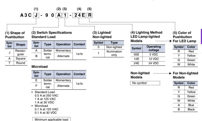
Momentary-action: Self-resetting Alternate-action: Self-holding
